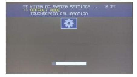
Keeping the finger on the screen the user have the possibility to repeat the touchscreen calibration.
