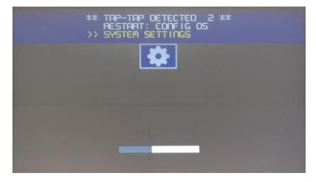
By keeping now the finger on the screen the "RESTART: CONFIG OS" option will remain selected and after 5 seconds the panel will reboot in the ConfigOS recovery mode (see).
